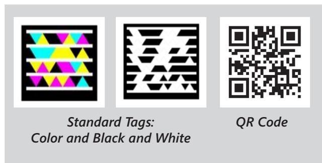
Tag barcodes and QR Codes are generated in vector graphics format so that they can be infinitely scaled from small to large yet maintain a crisp visual appearance. Standard Tag barcodes use a space-efficient set of color or black-and-white
